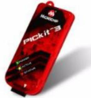
**Note: The PICKit 3 In-Circuit Debugger/Programmer is NOT a production programmer. It should be used for development purposes only.**
