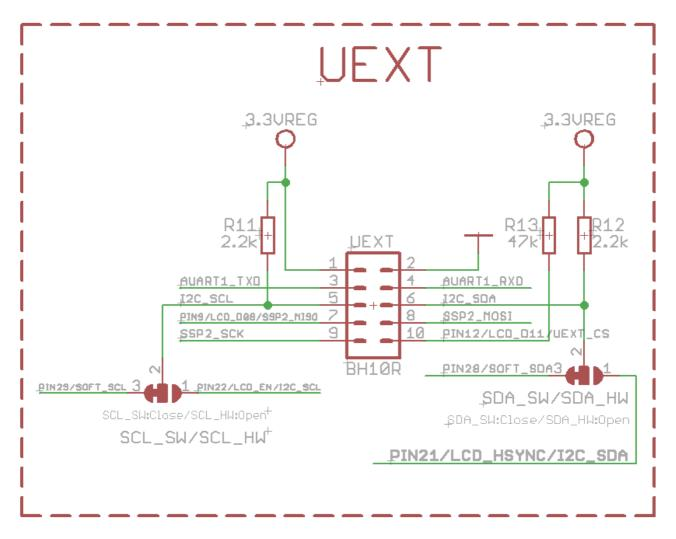
\*Note the two jumpers PIN29/SOFT\_CL – PIN22/LCD\_EN/I2C\_SCL, and PIN28/SOFT\_SDA3 – PIN21/LCD\_HSYNC/I2C\_SDA which by default are set to a software SPI. They can be used to set the whole UEXT to a hardware SPI.
