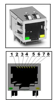
The two leds on the front side of the LAN connector show the state of the Ethernet. The meaning behind the different states can be found in the table below:
