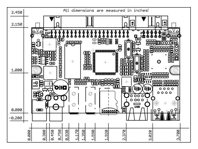
The three highest elements on the board in order from the tallest to the shortest are: inductor L2; USB host connector; Ethernet/LAN connector.
