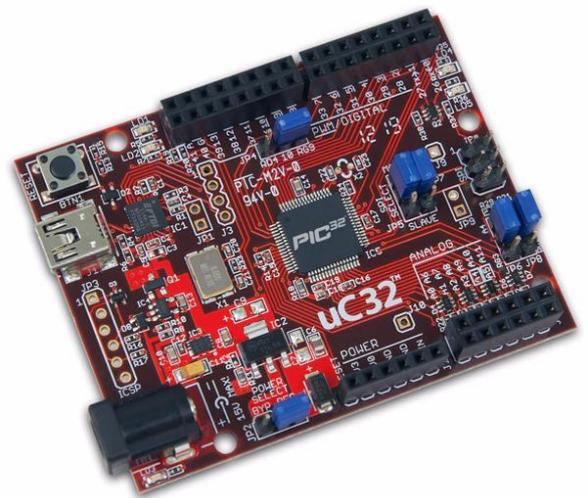
The uC32 board takes advantage of the powerful PIC32MX340F512 microcontroller. This microcontroller features a 32-bit MIPS processor core running at 80MHz, 512K of Flash program memory and 32K of SRAM data memory.
