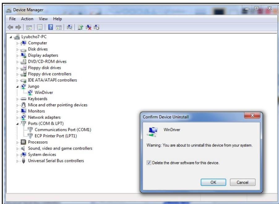
9. Install the new drivers corresponding for your needs (the picture below shows how to install the LibUSB drivers over the Jungo ones – you have to browse to the LibUSB folder and install anyway)
