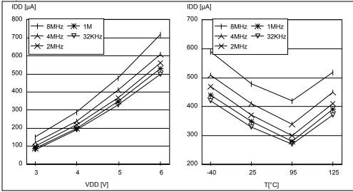
Figure 39. Typical  $I_{\text{DD}}$  in WAIT vs  $f_{\text{CPU}}$  and Temperature for OTP devices with option bytes programmed to 00H
