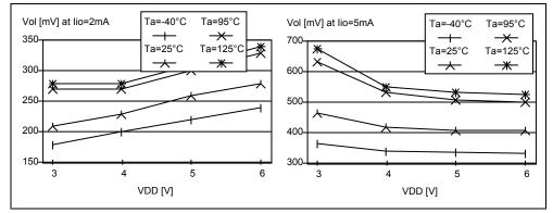
Figure 61. Typical V<sub>OL</sub> vs V<sub>DD</sub> (high-sink I/Os)
