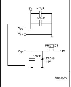
Note: ZPD15 is used for overvoltage protection
