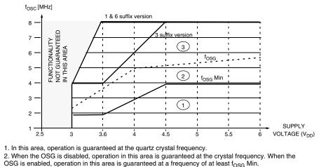
3. When the OSG is enabled, access to this area is prevented. The internal frequency is kept at  $f_{OSG}$  with the OSG is enabled, access to this area is prevented. The internal frequency is kept at  $f_{OSG}$ .
