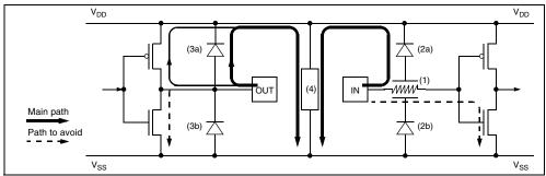
Figure 54. Negative Stress on a Standard Pad vs. V<sub>DD</sub>
