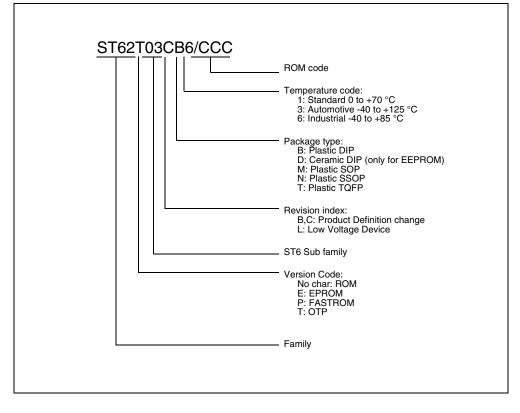
Figure 72. ST6 Factory Coded Device Types
