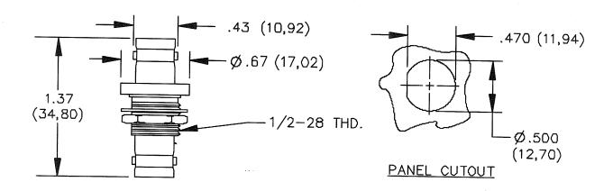
BNC Body is isolated from the mounting flange
