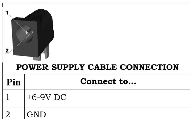
Note: If you want to use the board with external power supply, you have first to switch to UART mode when your board is connected to the USB (USB HID or USB CDC mode).
