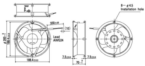
Reference dimensional diagram for installation holes (unit:mm)
