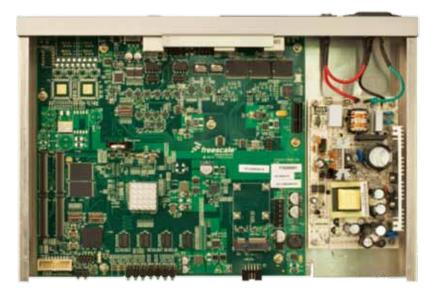
The P1024RDB features 1 GB unbuffered DDR3 SDRAM, 16 MB NOR flash and 32 MB NAND flash, with boot options. The board supports six Gigabit-capable ports, four ports from an L2 switch, one port via an SGMII PHY and one port via an RGMII PHY, as well as two USB 2.0 ports, four FXS ports and one FXO port.
