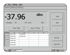
The YOPM, a PCMCIA-based Optical Power Meter, supports all your optical power measurement needs. It measures all common telecommunication wavelengths from 850 nm to 1625 nm. Easy saving of measurement data makes this an ideal tool for documenting networks.
