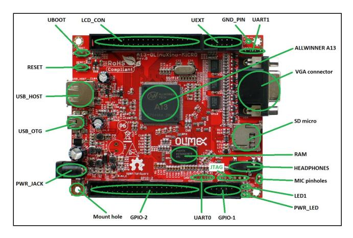
The picture above shows the initial revision B of A13-OLinuXino-MICRO.
