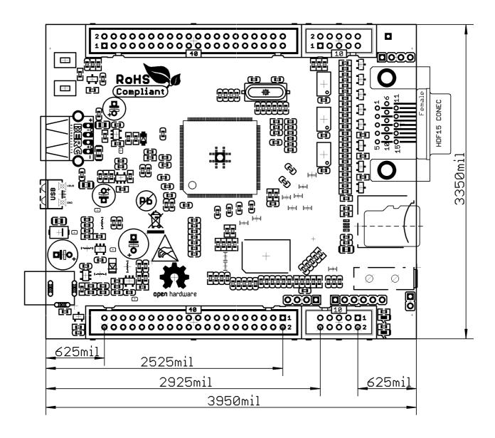
The three highest elements on the board in order from the tallest to the shortest are: the VGA connector—560mils, capacitor C102 —550mils, capacitor C53 —500mils. Note that those heights include the PCB.
