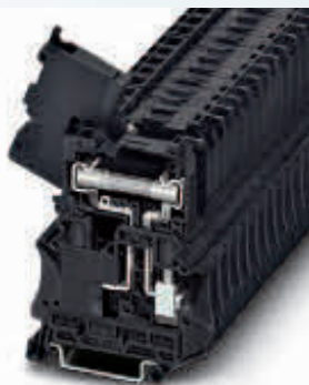
6 (10) mm 2 , 10 A, lever-type fuse terminal block for 6.3 x 32 mm cartridge fuses
