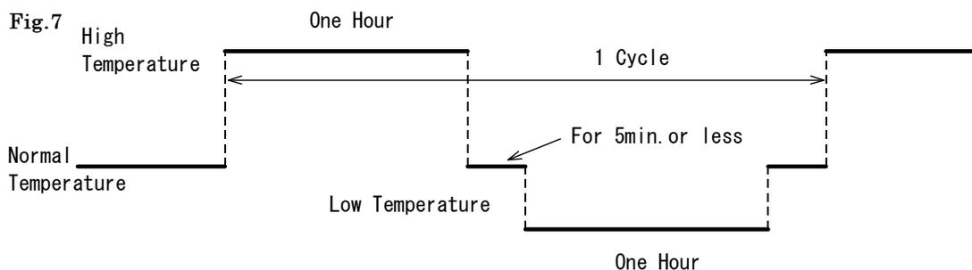
Thermostatic chamber temperature is set at 125°C as the high temperature and -40°C as the low temperature
