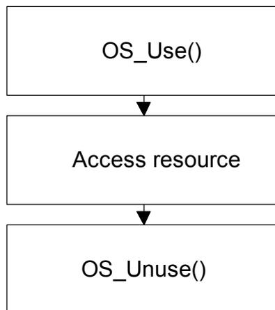
A resource semaphore contains a counter that keeps track of how many times the resource has been claimed by calling `OS_Request()` or `OS_Use()` by a particular task. It is released when that counter reaches 0, which means the `OS_Unuse()` routine has to be called exactly the same number of times as `OS_Use()` or `OS_Request()`. If it is not, the resource remains blocked for other tasks.
