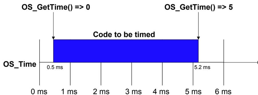
The call to `OS_Timing_Start()` calculates the starting value at 5,000 cycles, while the call to `OS_Timing_End()` calculates the ending value at 52,000 cycles (both values are kept track of internally). The measured execution time of the code in this example would therefore be  $(52,000 - 5,000) = 47,000$  cycles, which corresponds to 4.7 ms.
