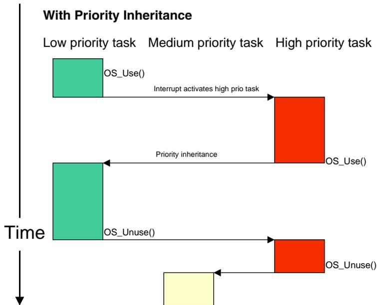
With priority inheritance, the low priority task inherits the priority of the waiting high priority task as long as it holds the resource semaphore. The lower priority task is activated instead of the medium priority task when the high priority task tries to claim the semaphore.
