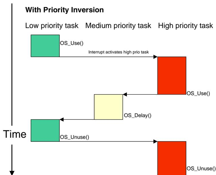
The low priority task claims the semaphore with `OS_Use()`. An interrupt activates the high priority task, which also calls `OS_Use()`.
