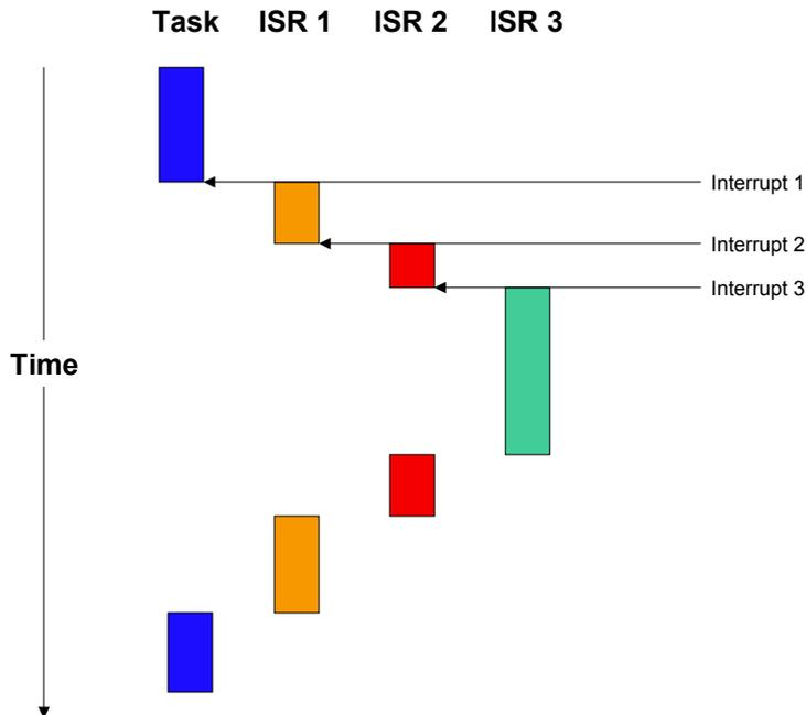
For applications requiring short interrupt latency, you may re-enable interrupts inside an ISR by using `OS_EnterNestableInterrupt()` and `OS_LeaveNestableInterrupt()` within the interrupt handler.
