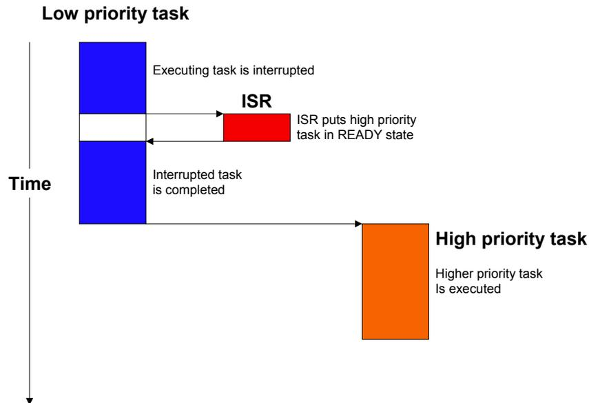
A pure cooperative multi-tasking system has the disadvantage of longer reaction times when high priority tasks become ready for execution. This makes their usage in embedded systems uncommon.
