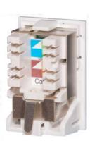
The Connectix Category 6 FTP LJ6C Module provides the performance needed for present and next generation data communications networks and applications, including Gigabit Ethernet, with the added benefit of shielding to minimise the risk of EMI. The use of next generation components and specially designed boards allow a bandwidth of 250MHz to be achieved in a shielded package.
