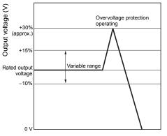
The values shown in the above diagram is for reference only. Note: Do not turn ON the power again until the cause of the overvoltage has been removed.
