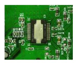
Sound Terminals<sup>™</sup> are high performance, integrated single chips capable of digitally processing and amplifying audio signals maintaining a fully digital format from source to speaker, thus reducing the BOM, the design costs, the footprint area and at the same time improving the clarity of the sound.
