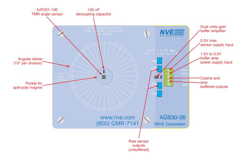
Each of the four sensor elements contains two magnetic layers: a "pinned," or fixed direction layer; and a movable-direction, or "free" layer. Internal sensor pairs are  $90^{\circ}$  out of phase to provide quadrature outputs.
