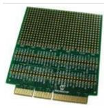
The Prototype PICtail Plus Daughter Board allows a designer to breadboard their solution easily for evaluation on an Explorer 16 Evaluation Board using PIC24 MCU or dsPIC33 DSC. This board is an 8 x 8 cm board with a card-edge connection that allows it to be plugged directly into the PICtail Plus expansion socket. The breadboard area provides access to all of the processor pins as well as a generous prototyping area. AC164126 contains three blank Prototype PICtail Plus Daughter Boards.
