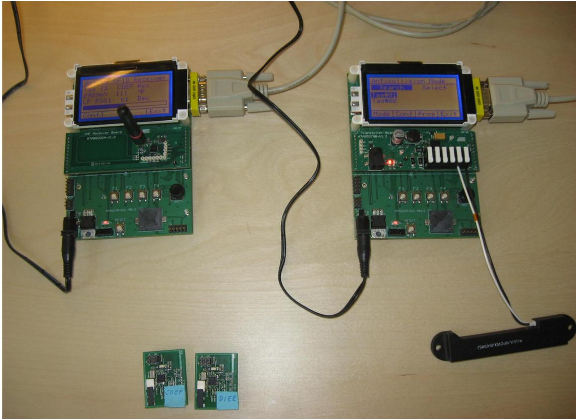
The null modem cable provides a bidirectional serial interface between the LF and the RF modules of the base station. It is used for synchronization of the LF and RF channel data in anticollision mode and also transfers the received data back to the LF emitter module which is acting as the master. This received data is buffered and held for recovery and displayed on the LF emitter module display.
