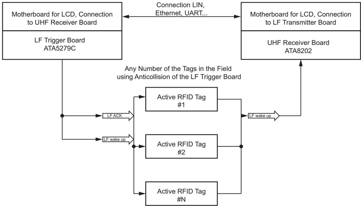
**Figure 1-2. Atmel ATA6286-EK3 Development Kit**
