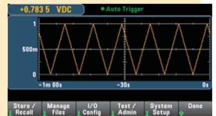
The engineers set up the Agilent 34461A to measure the on/off output voltage of the detector circuit and displayed the results using the histogram mode. At frequencies below one Hertz, the display clearly showed a binary distribution, which was the desired result.
