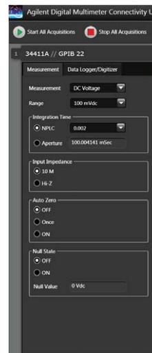
Figure 2. DCV setup
