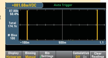
However, they found that for higher frequencies, which occurred when they waved a hand across the solar panel, the circuit exhibited an anomaly that caused an intermediate output value. This anomaly clearly interfered with the proper output charging operation.
