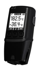
The EL-GFX-DTC standalone USB data logger measures and stores up to 252,928 temperature readings from two J, K, or T-type thermocouple inputs at a resolution of 0.1°C. Using the Windows control software (available as a free-download from www.easylogusb.com), users can quickly set up the data logger and view downloaded data by connecting the device to the PC's USB port using the supplied cable.
