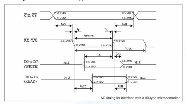
AC timing for interface with a 80-type microcontorller at VDD=5 volts VDD = 5 V  $\pm 10\%$ ; VSS = 0 V; Tamb = -20 % to  $\pm 75\%$ .
