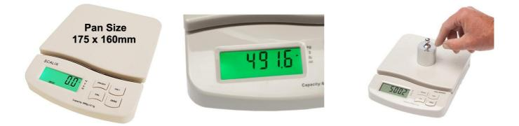
These precision weighing balances are have an impact-resistant ABS plastic case and weighing pan, a splash-proof protective cover and non-slip rubber feet. The balance can be either battery or mains powered.
