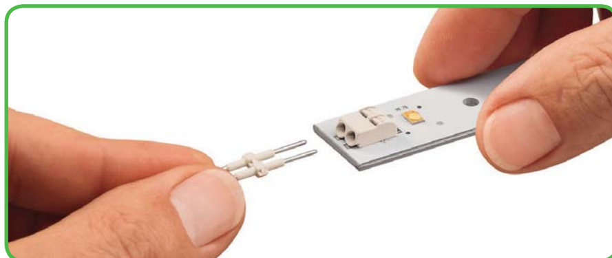
Inserting the connecting link into terminal block.
