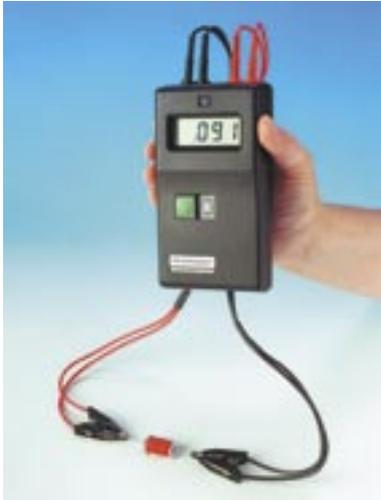
This instrument is a portable digital meter to measure low resistances over the range 0.001Ω to 200Ω. A high degree of accuracy is achieved by utilising a four terminal input to eliminate errors caused by test lead length.
