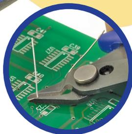
Shearing action of blades produces a clean precise cut with less effort.
