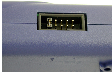
Figure 3-13: Jumper Settings for Target Power Connection via Power In and Power Out Jacks Of Cyclone PRO
