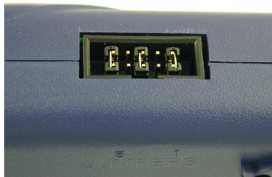
Figure 3-21: Jumper Settings For Power IN Jack And MON08 Header Pin 15
