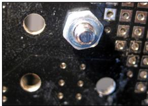
Then you can fasten the four 25mm M3 spacer bolts one after the other with the M3 nuts in the mounting holes on the main board as shown on the picture.
