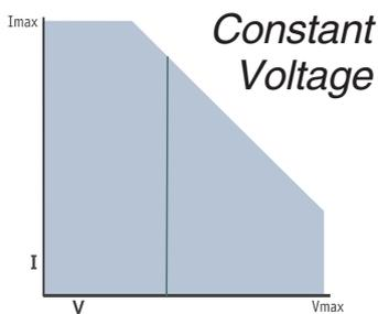
Constant voltage mode is used for load testing of constant current power supplies. The unit operates as a high power shunt regulator.
