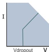
If the voltage applied to the load falls below a preset level, the load current is rapidly reduced to zero.
