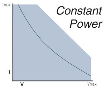
Constant power mode simulates a load whose power consumption is independent of the applied voltage. This is true of many types of equipment that incorporate switchmode regulators.
