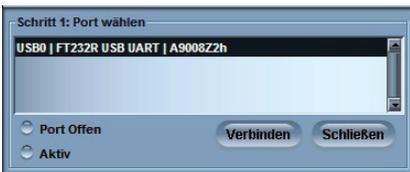
Select the USB port. As long as no other USB->Serial Adaptor with FTDI controller is connected to the PC, you will see only one single entry that you have to select.
