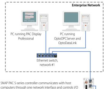
This diagram shows multiple Opto 22 SNAP I/O units connected together over an Ethernet network and controlled by a SNAP PAC S-series controller running a control strategy. The controller is also connected to a larger, separate enterprise Ethernet network to provide data to two PCs running Opto 22's PAC Display HMI software and OptoOPCServer.
