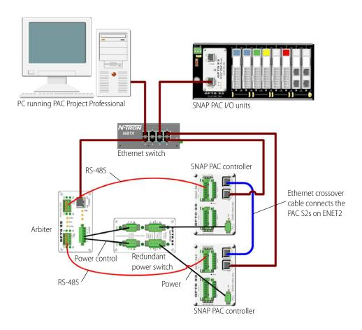
In this diagram, two S-series controllers are operating redundantly. One is the active controller, while the other acts as a backup, ready to take over should the first one fail.
