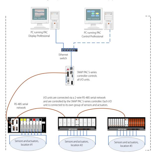
This diagram shows a SNAP PAC S-series controller connected to multiple Opto 22 serial-based I/O units over an RS-485 serial network. The controller is also connected to a larger, separate enterprise Ethernet network to provide process data to a PC running Opto 22's PAC Display HMI software.
