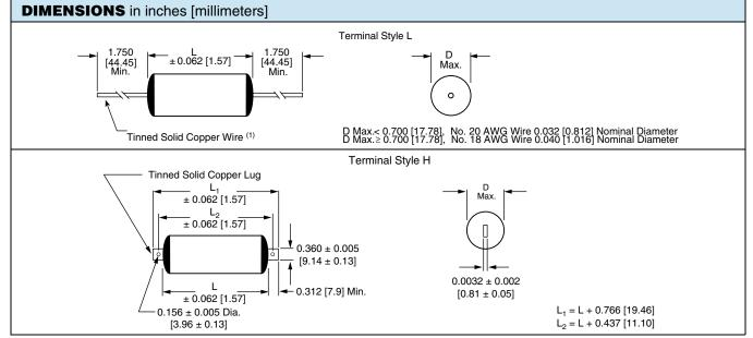
Note (1) Leads to be within ± 0.062" [1.57 mm] of center line at egress but not less than 0.031" [0.79 mm] from edge (Terminal Style L only).
