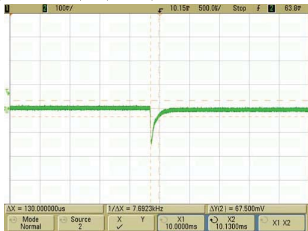
Step Load Transient Response (Slew=1A / \mu Sec., Vin=48V, Clad=0, Iout=22.5A to 15A)
