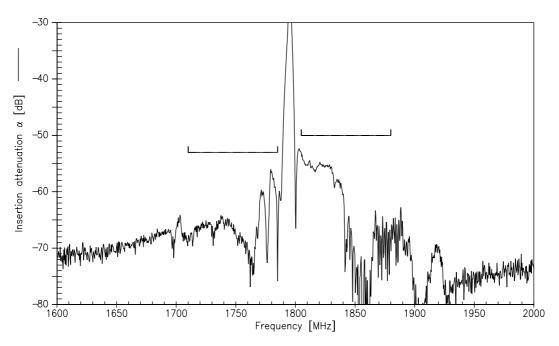
Frequency Response TX-RX (differential mode, wideband)
