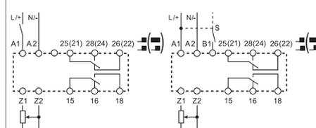
Wiring diagram (without control signal)
