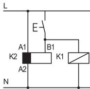
• Possible to control an external load, such as another relay coil or timer, connected to the control signal terminal B1.
