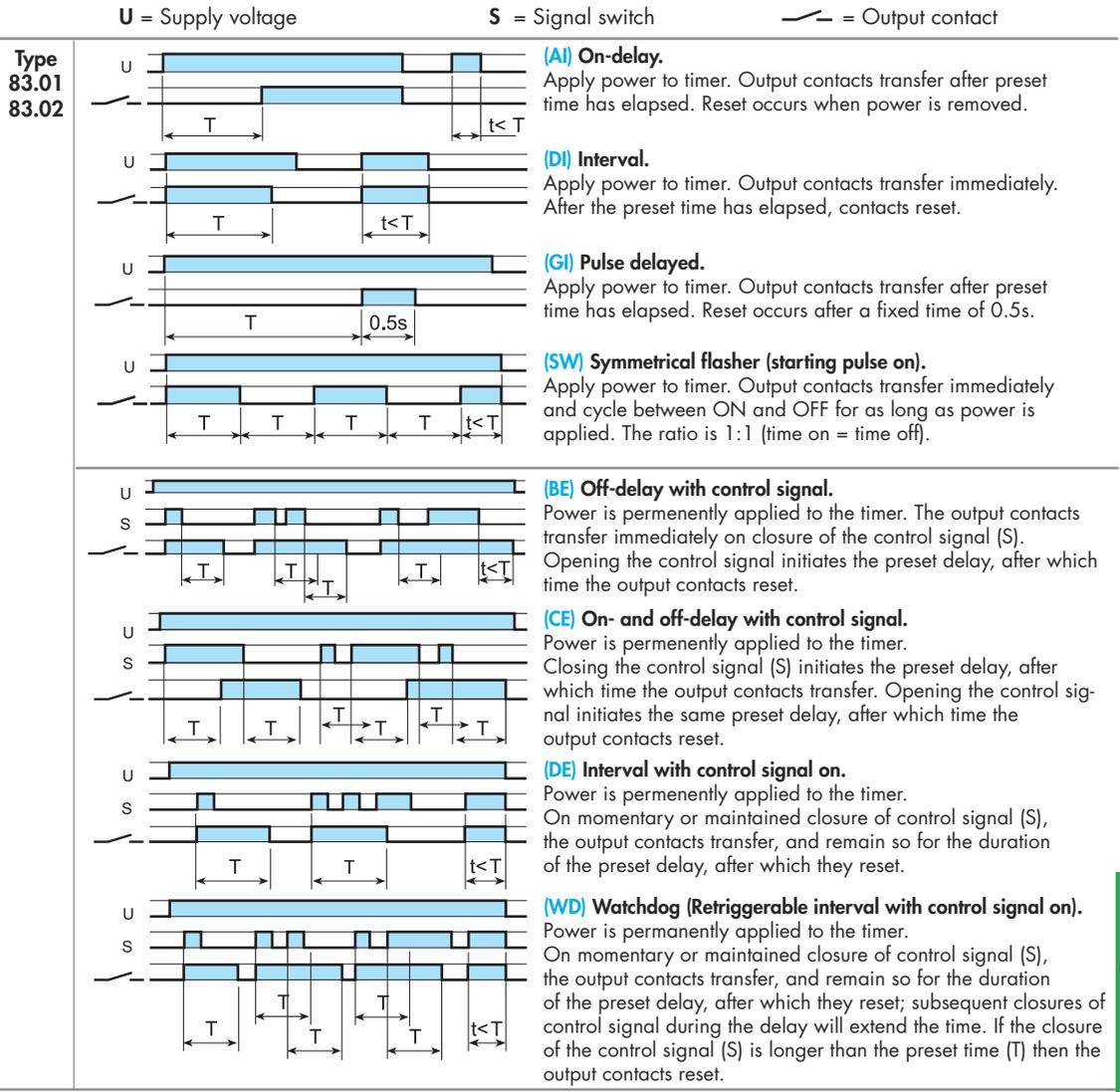
NOTE: The timing function must be set when the timer is de-energised. Or for the 83.02, when the contact mode selector is in the OFF position.
