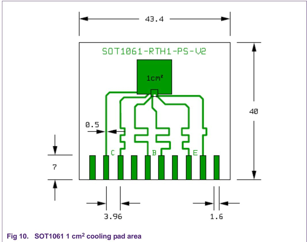
Fig 10. SOT1061 1 cm<sup>2</sup> cooling pad area
