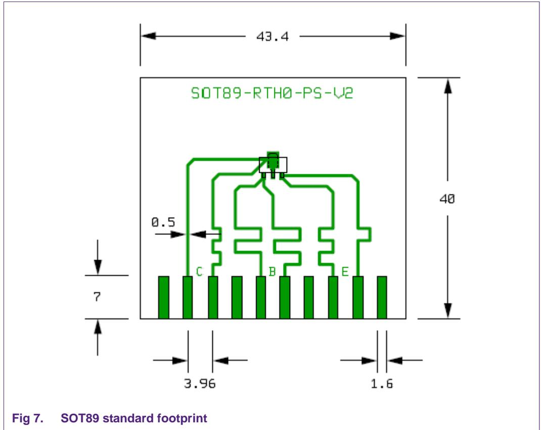
Fig 7. SOT89 standard footprint
