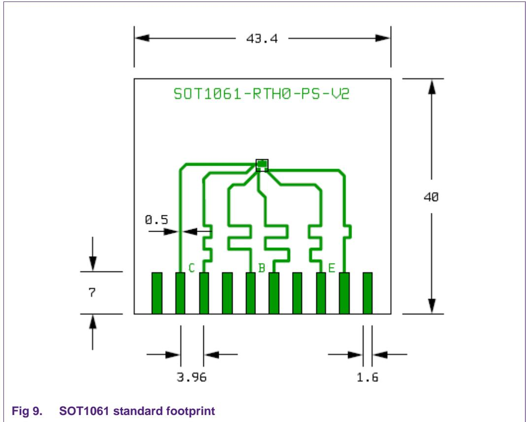
Fig 9. SOT1061 standard footprint
