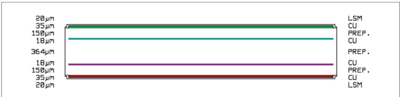
Fig 3. Layer stack of modified  $R_{th}$ -PCBs
