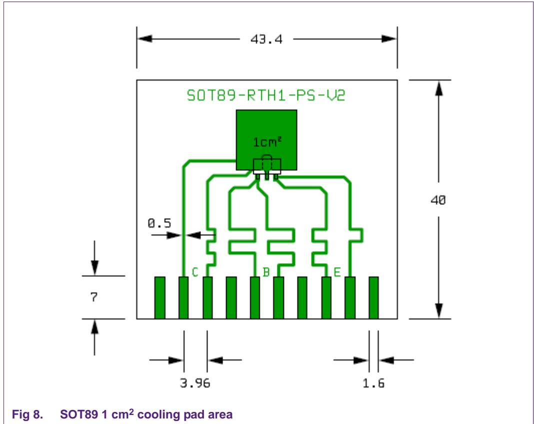
Fig 8. SOT89 1 cm<sup>2</sup> cooling pad area
