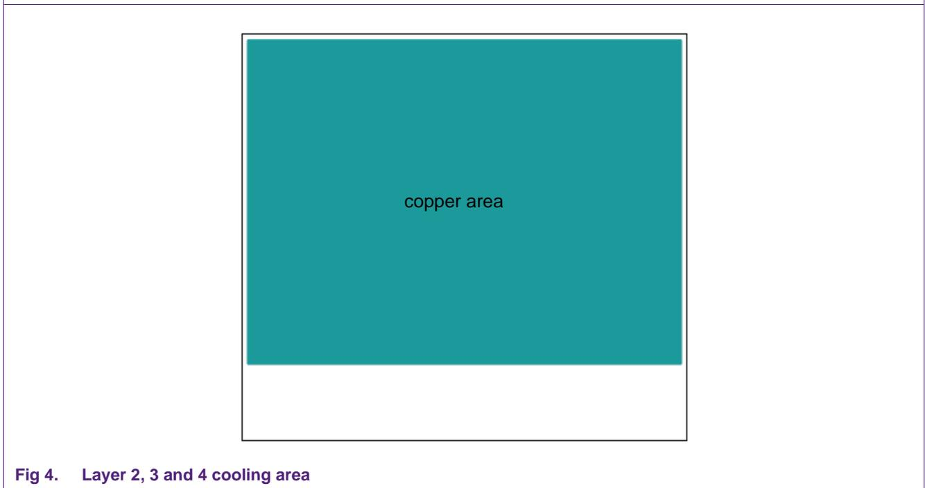
Fig 4. Layer 2, 3 and 4 cooling area
