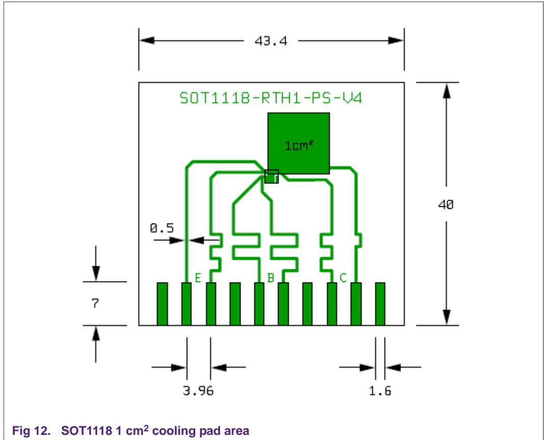
Fig 12. SOT1118 1 cm<sup>2</sup> cooling pad area
