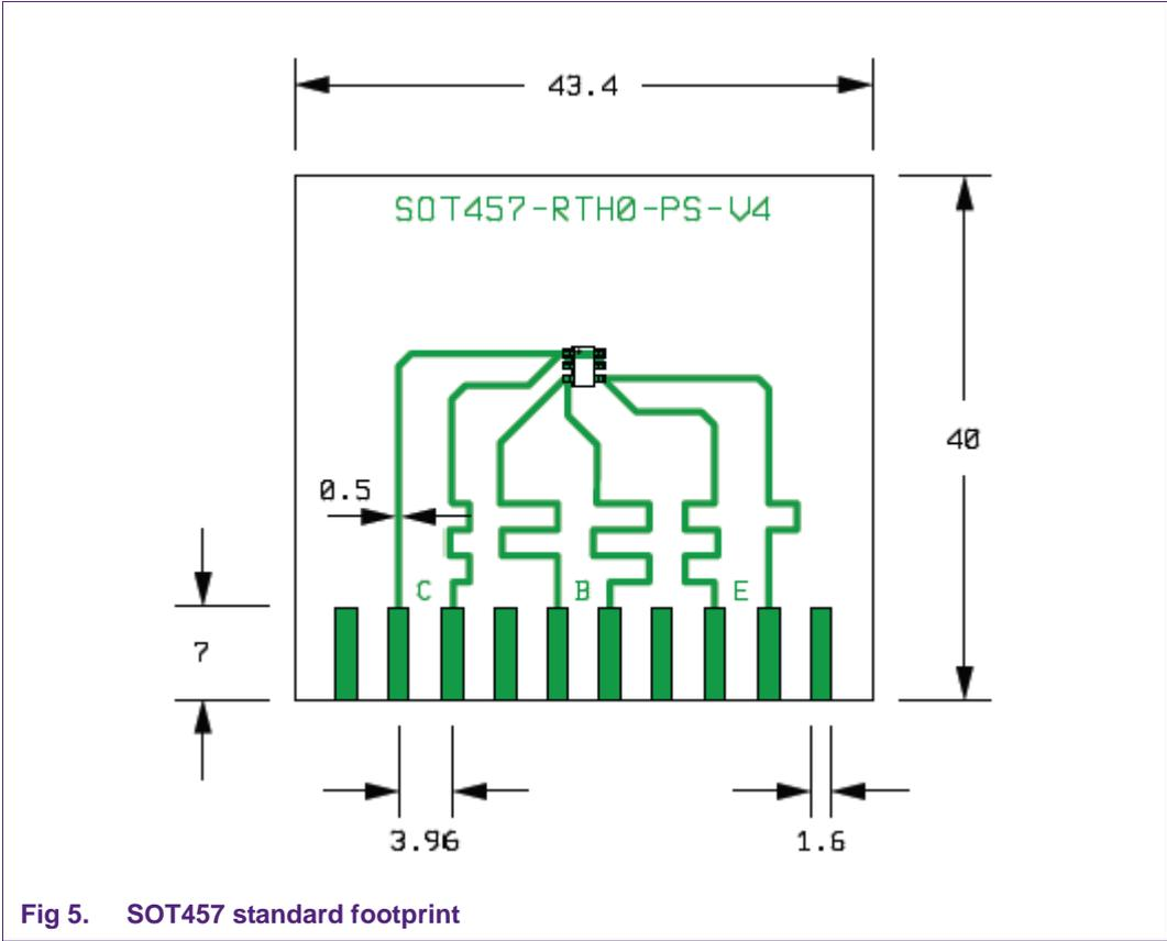
Fig 5. SOT457 standard footprint
