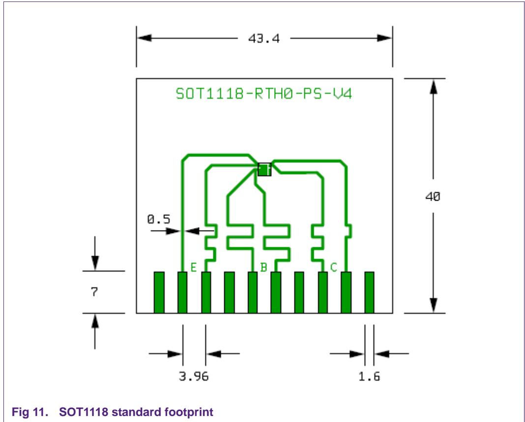
Fig 11. SOT1118 standard footprint
