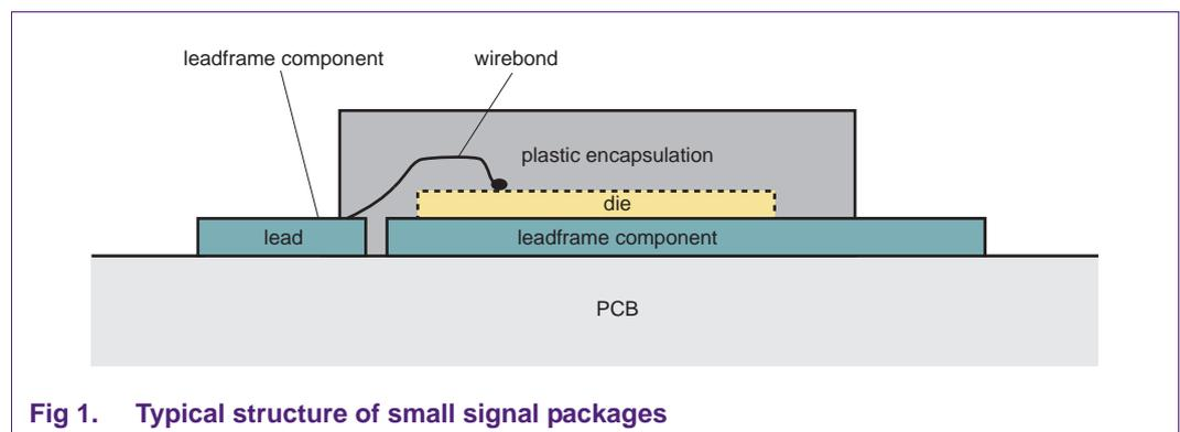
Fig 1. Typical structure of small signal packages
