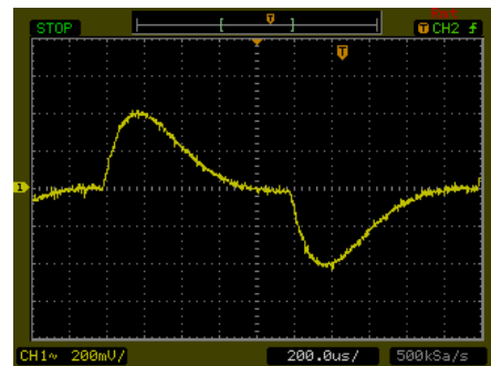
Transient Response to Dynamic Load Change from 100% to 75% of Full Load ; V_{in} = V_{in\ nom}
