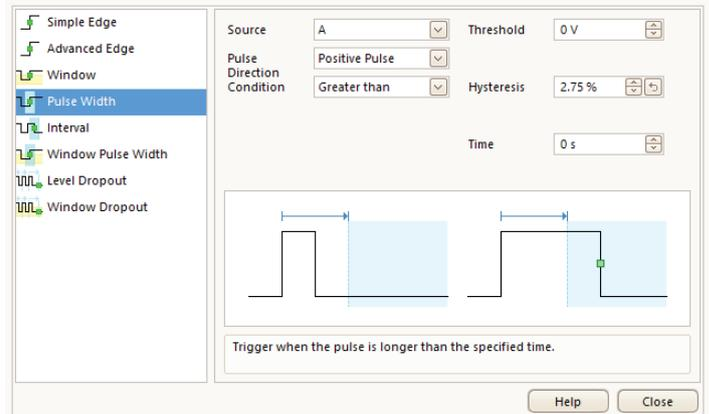
For over 20 years Pico have been pioneering the use of full digital triggering using the actual digitized data. This reduces trigger errors and allows our oscilloscopes to trigger on the smallest signals, even at the full bandwidth. All triggering is digital, resulting in high threshold resolution within programmable hysteresis and optimal waveform stability.
