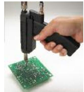
Through hole desoldering with the MX-DS1 hand-piece.
