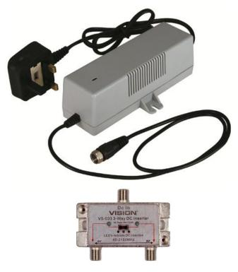
V5-EVO systems are designed to be flexible for small, medium and large installations. Each design may have different powering requirements due to the nature and layout of the building. V5-034 switch-mode-power-supply is designed to provide up to 2.5A at 18V which is enough to power even the largest of installations with as many as 40 x EV5-532 multiswitches connected together. That's a total of 1,280 subscriber cables!
