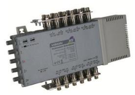
multiswitches for smaller to medium cascaded networks. These mains-powered multiswitches can be used to power up to six line powered multiswitches and an LNB. EV5-xxxM will power a Quattro LNB via the horizontal and vertical inputs at up to 650mA max. Power is provided from the built-in switch-mode power supply.
