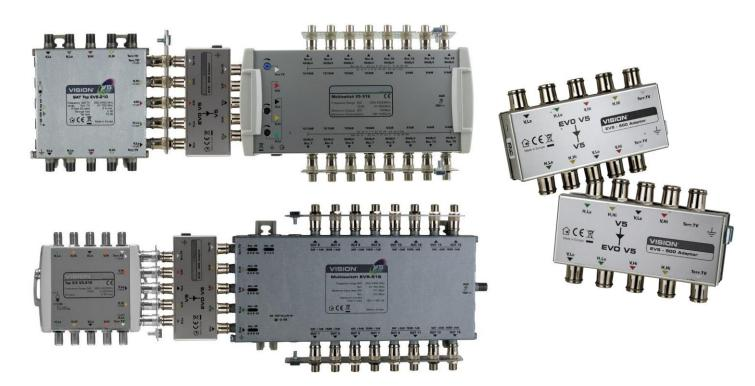
The new EV5 has wider pitched input connectors than the original V5 components to improve access and enhance performance. For improved isolation between terrestrial and satellite as well as between all satellite polarities, the order of connectors has been changed. To avoid making short interconnecting leads use EV5-500 adapter.
