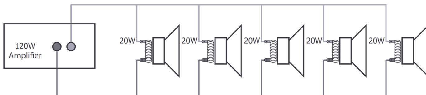
A 100V line speaker system can comprise of many speakers connected together. The determining factor for how many speakers can be used on a single amplifier is the power rating. For most purposes, it is advised to connect as many speakers as needed with a combined wattage of no more than 90% of the amplifier's output power rating.
