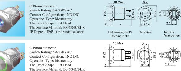
The Surface Material: BS/SS/B/BLK IP Degree: IP65 (IP67 Made To Order) Latching is 39.
