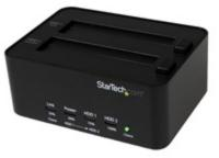
The SATDOCK2REU3 USB3.0 Standalone Duplicator and Eraser Dock lets you connect your 2.5in/3.5in SATA HDDs or SSDs through SuperSpeed USB 3.0, with the ability to swap drives in and out as needed. The dock also functions as a standalone drive duplicator and eraser – an efficient and versatile solution for external drive management.
