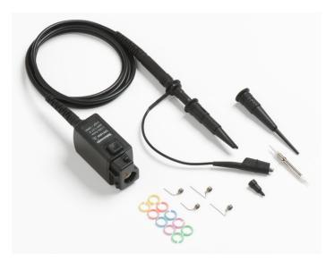
The TPP1000, TPP0500 and TPP0502 models are high-bandwidth, general-purpose probes from Tektronix that offer breakthrough specifications previously unrealized in this product class. Designed for use with Tektronix MSO/DPO4000B and MSO/DPO5000 Series oscilloscopes, these probes provide up to 1 GHz of analog bandwidth with less than 3.9 pF of capacitive loading.
