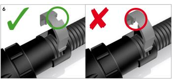
Orientate the oval retaining clip as illustrated and locate it in the slot as shown.
