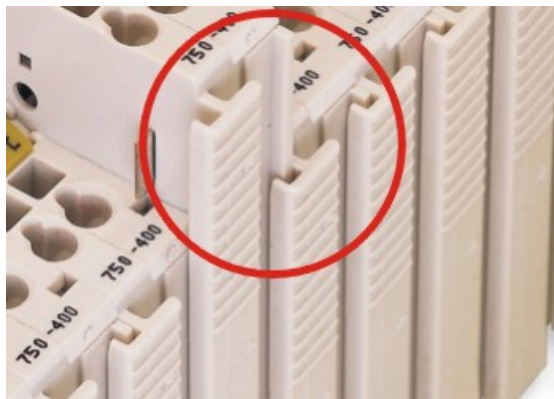
Figure 28: Insert I/O module
