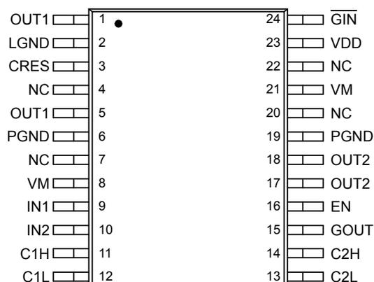
**Figure 3. 17510 Pin Connections**
