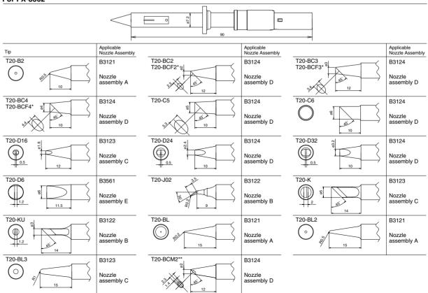
\* Tinned on the soldering surface only. \*\* The part number T20-BCM2 is not available for sale or use in the U.S.A.
