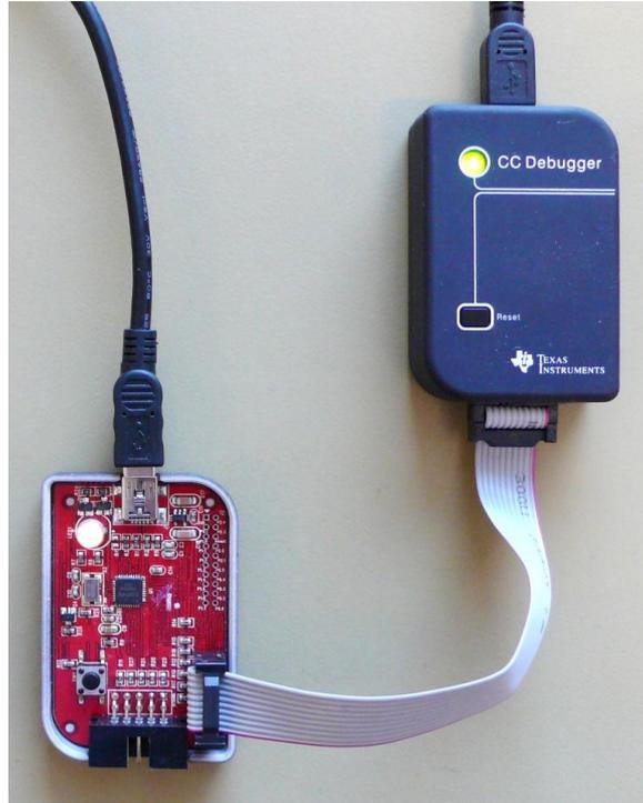
**Figure 18 - Programming the bootloader on the CC Debugger using another CC Debugger**
